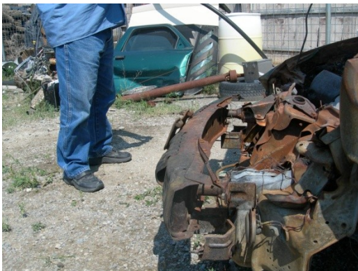
Figure 3. No crush damage by major load carrying components.
