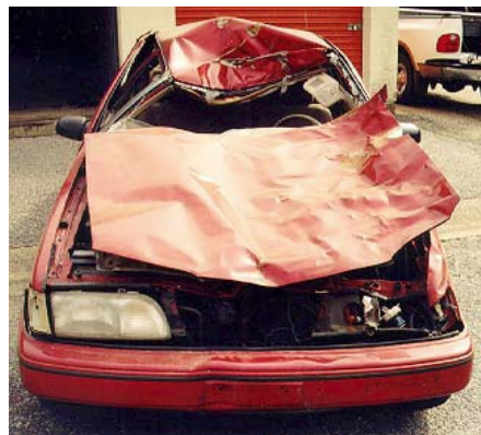
Figure 4. 1991 Hyundai Sonata cow crash damage.
