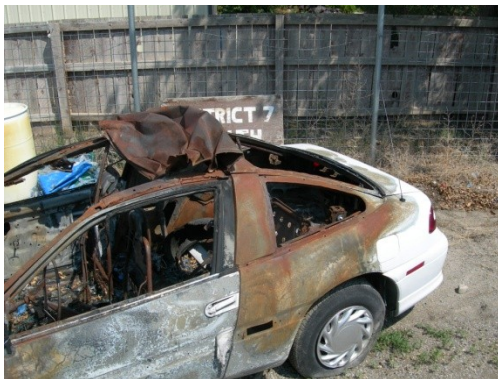
Figure 2. Peeling back of roof panel.
